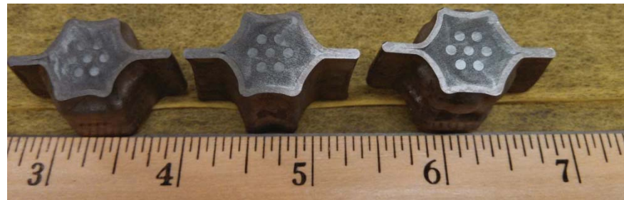
Above/Below: 7 channel WUO 2 fuel element post HIP and cross sections
