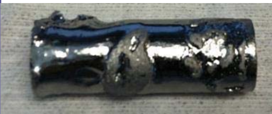
Above/left: Pure W sample post shakeout run 2. Sample reached melting point (3695K) and was held in place by the BN insulator.
