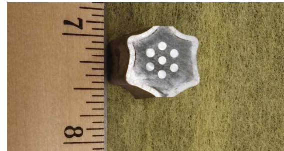
Above/Below: 7 channel WUO 2 fuel element post HIP and cross sections
