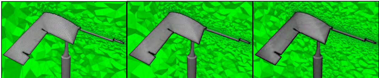
Figure 5. Volume grid through right-wing control surface of DLR-F19 CS20. Left to right: G1.20, G2.20, G3.30.
