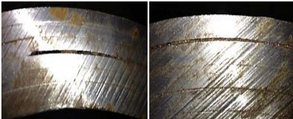
Figure 7.2.4-6. Corrosion between Layers on MSFC LPV V-32
