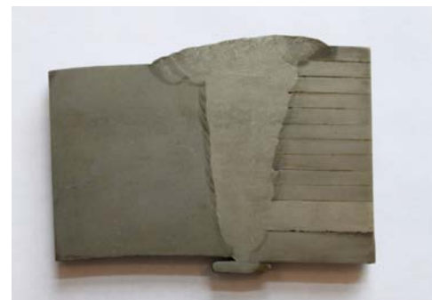
(a) Figure 5.0-2. Cross-sectional Diagram of LPV ((a) monolithic head and (b) cross section of actual vessel)
