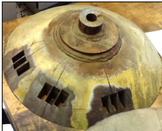
Figure 7.2.1.2-3. V0032-1 Sectioned for Metallographic Microstructural Examination for Determining Material Orientation
