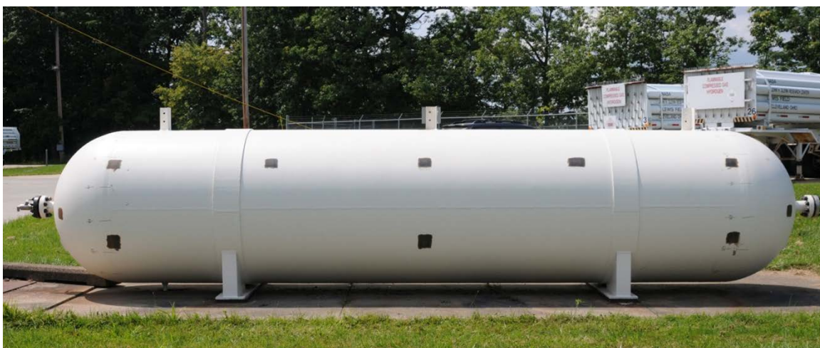
Figure 7.2.3.3-1. Test Pressure Vessel Cleaned and Painted White (black squares on the vessel are unpainted areas to accommodate AE sensors)
