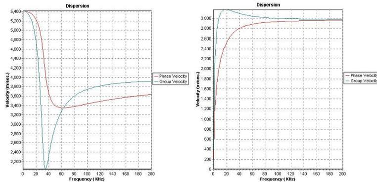
Dispersion curves for a 2.75 inch thick steel plate. The extensional mode curve is on the left, flexural mode curve is on the right [Ref 1, Fig 4]
