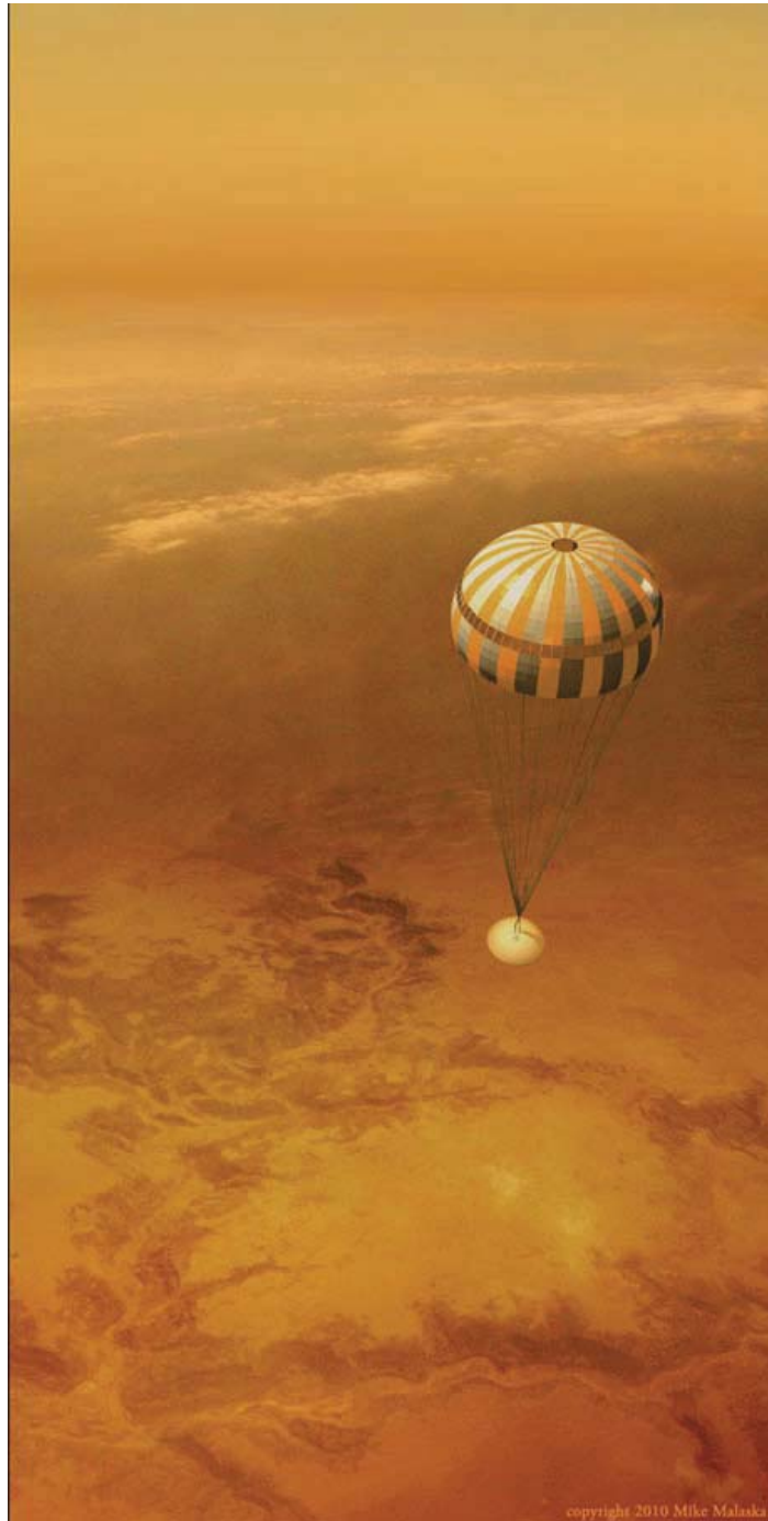
Fig. 31 An artist's conception of the parachuted descent portion of the AVIATR EDD sequence
