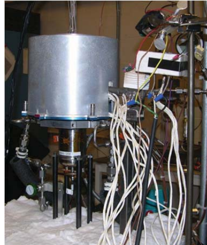
Figure 9. VCHP/ASC-1 HS with insulation.
