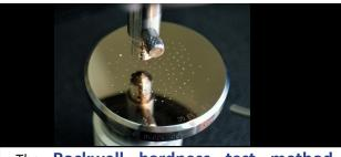
The Rockwell hardness test method consists of indenting the test material with a diamond cone or hardened steel ball indenter. The permanent increase in depth of penetration, resulting from the application and removal of the additional major load, is used to calculate the Rockwell hardness number.
