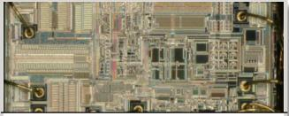
**Destructive physical analysis** is a systematic approach to disassemble a component, electronics board, part, etc. to evaluate it down to the basic material and construction level.
