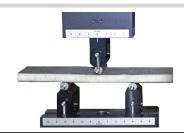
**Bend testing** is a procedure to determine the relative ductility of metal that is to be formed (usually sheet, strip, plate or wire) or to determine soundness and toughness of metal (after welding, etc.) The specimen is usually bent over a specified diameter mandrel. The four general types of bends are: free bend, guided bend (ASTM E190), semi-guided bend (ASTM E290), and wrap-around bend.
