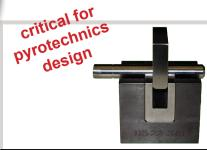
**Shear testing** is accomplished by exerting pressure (shear force) in the transverse plane of the sample until shear failure occurs.
