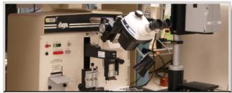
**Terminal strength testing** involves forces applied consisting of direct axial, radial or tension pulls, twist, bending torsion, and the torque exerted by the application of nuts or screws on threaded terminals.
