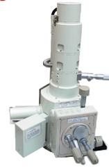
The **scanning electron microscope (SEM)** has many advantages over traditional microscopes. The SEM has a large depth of field, which allows more of a specimen to be in focus at one time. The SEM also provides higher resolution.
