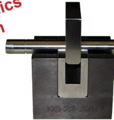
**Shear testing** is accomplished by exerting pressure (shear force) in the transverse plane of the sample until shear failure occurs.
