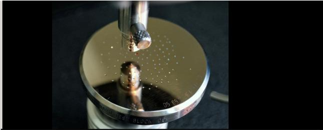
The **Rockwell hardness test method** consists of indenting the test material with a diamond cone or hardened steel ball indenter. The permanent increase in depth of penetration, resulting from the application and removal of the additional major load, is used to calculate the Rockwell hardness number.
