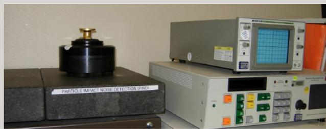
**Particle Impact Noise Detection** testing, known as PIND or PIN-D, is performed to detect loose particles inside a device cavity.
