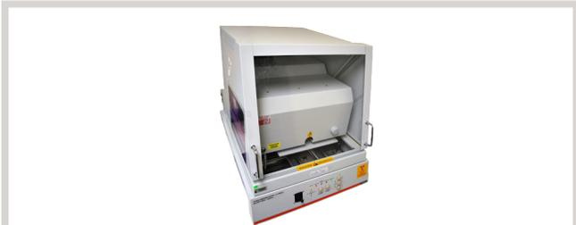
**X-ray fluorescence** is the emission of characteristic “secondary” (or fluorescent) X-rays from a material that has been excited by bombarding with high-energy X-rays or gamma rays. This technology is widely used for elemental analysis and chemical analysis, particularly in the investigation of metals, glass, and ceramics.
