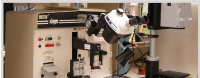
**Terminal strength testing** involves forces applied consisting of direct axial, radial or tension pulls, twist, bending torsion, and the torque exerted by the application of nuts or screws on threaded terminals.
