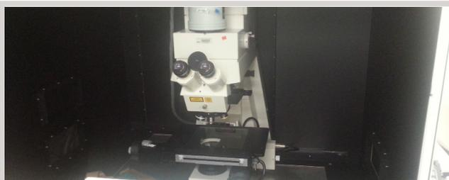
The purpose of the **emission microscopy** is to detect microcircuit failure sites by light emission leakages.
