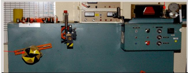
**Wire and cable testing** is performed by conducting multiple tests including spark testing, cold bend, dimensional, etc.
