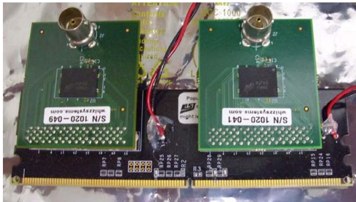
Figure 4.1-1: Adapter for connection of NEPP DDR2 individual DUT daughter cards.
