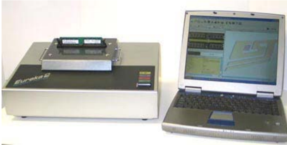
Figure 4.2-1: The Eureka 2 test system is an acceptance tester for DDR2 DIMMs.
