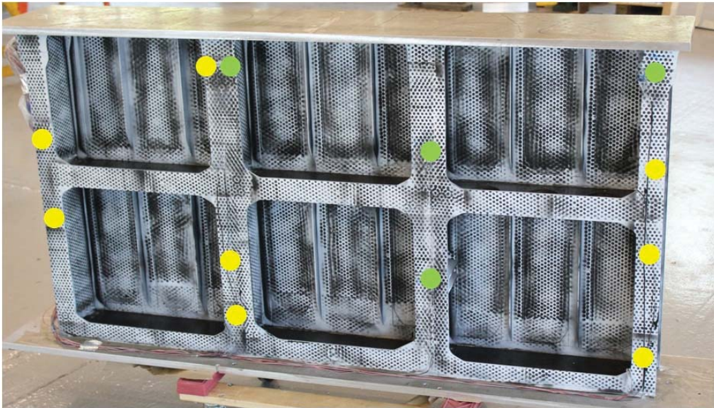
Figure 44. Pre-test photograph of the subfloor section highlighting strain gage locations.
