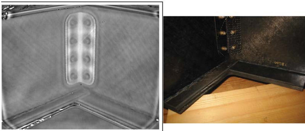
Figure A-31. Thermal inspection results for cruciform 2, rivet 3 bottom.
