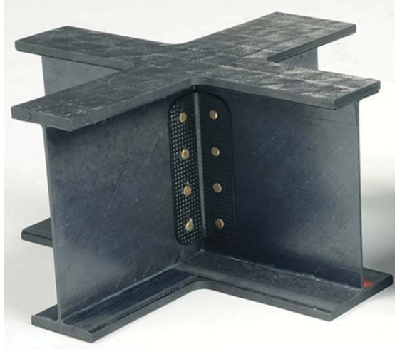
Figure 30. Photograph of a cruciform section test specimen.
