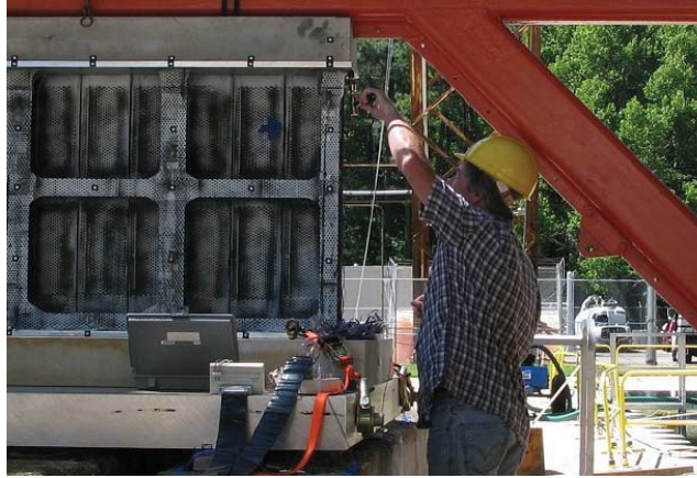
Figure 47. Tap excitation in vertical direction.
