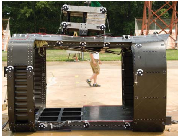
Figure 1. Post-test photograph of the SARAP TVA following the 2008 vertical drop test.
