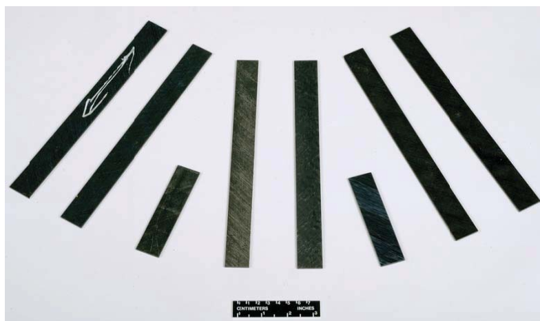
Figure 4. Sample set of extracted coupon specimens.
