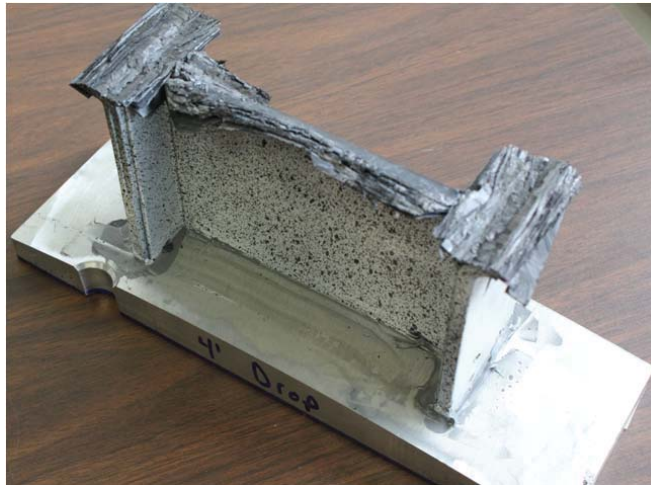
Figure 13. Post-test photograph of the I-beam tested at 4-ft drop height.
