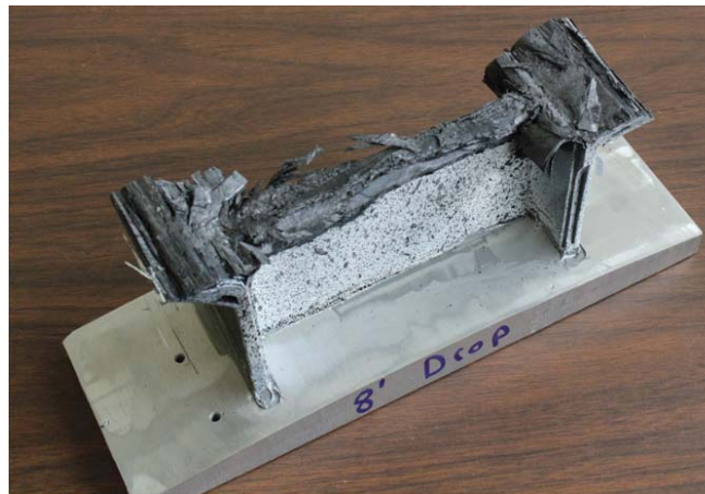
Figure 18. Post-test I-beam specimen following 8-ft drop test.
