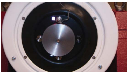
Figure 5.—Dummy mass attached to shaker armature.
