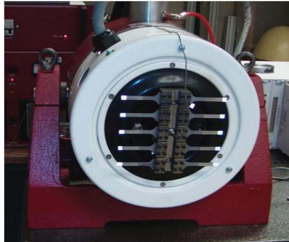
Figure 19.—Ten specimens mounted on armature.
