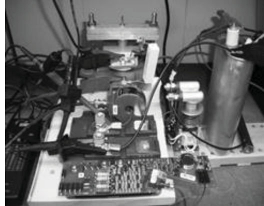
Figure 3: a) Double pulse test circuit schematic. b) Lab setup of double pulse test circuit.
