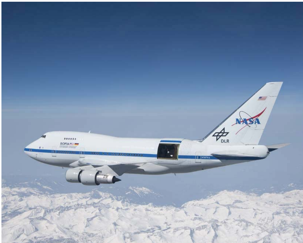
Figure 3. SOFIA cavity door system.
