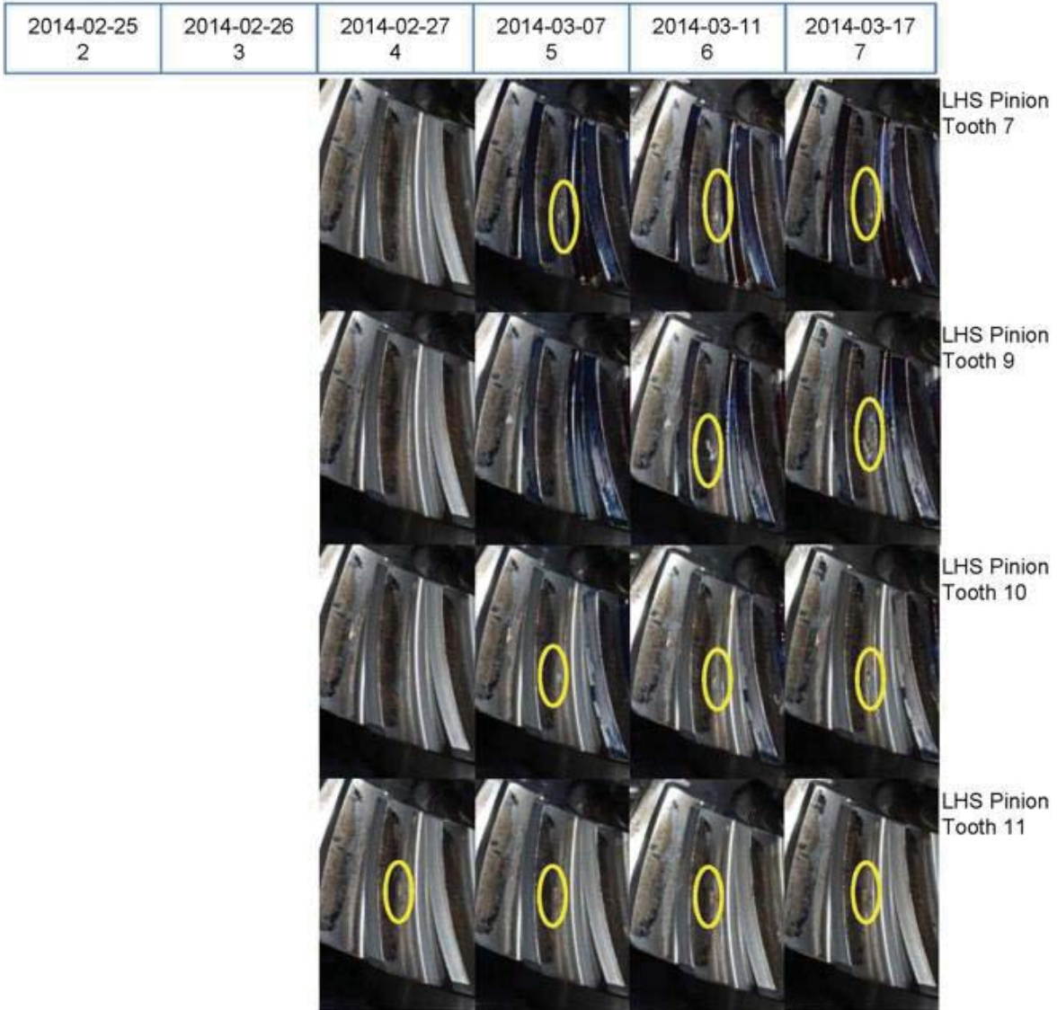
Figure A.1.9.—Test L2121R1919 pinion damage modes.
