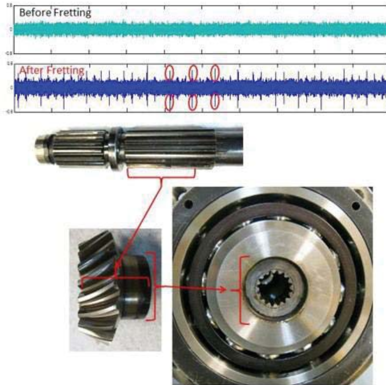
Figure 15.—Fretting of pinion in shaft.
