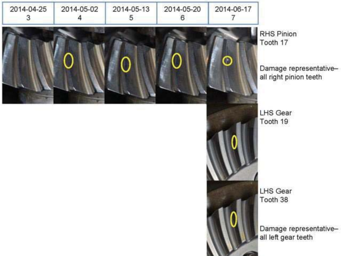
Figure A.1.12.—Test L3737R2424 damage modes.
