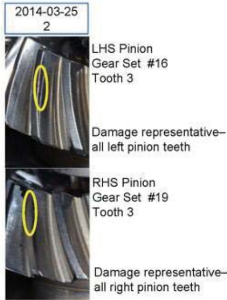
Figure A.1.11.—Test L1616R1919 pinion damage modes.
