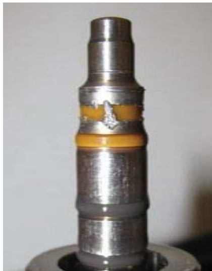
Figure 4.—Photograph of chip detector with captured debris.
