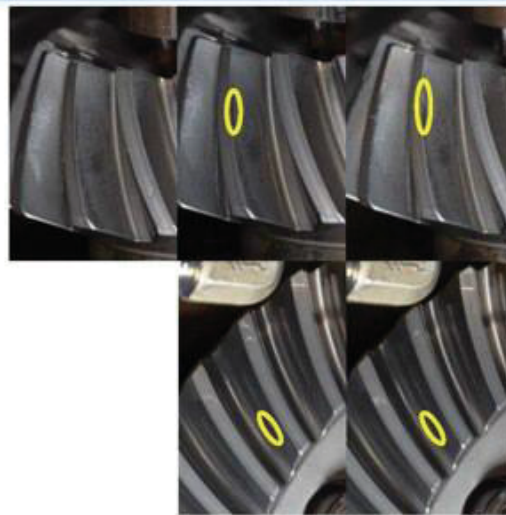
Figure A.1.15.—Test L4444R5252 damage modes.
