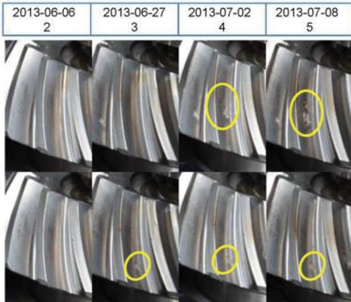
Figure A.1.3.—Test L1515R5050 pinion and gear damage modes.
