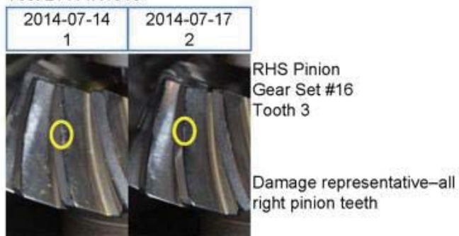
Figure A.1.14.—Test L1414R1616 damage modes.
