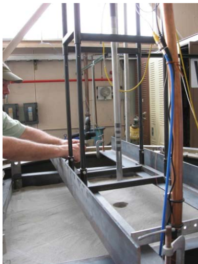
Figure 11.—The cone penetrometer on a fixed frame in phase 1.
