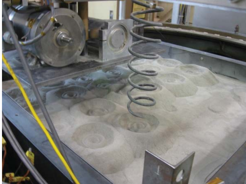
Figure 17.—The auger is shown tilling the soil at room conditions.
