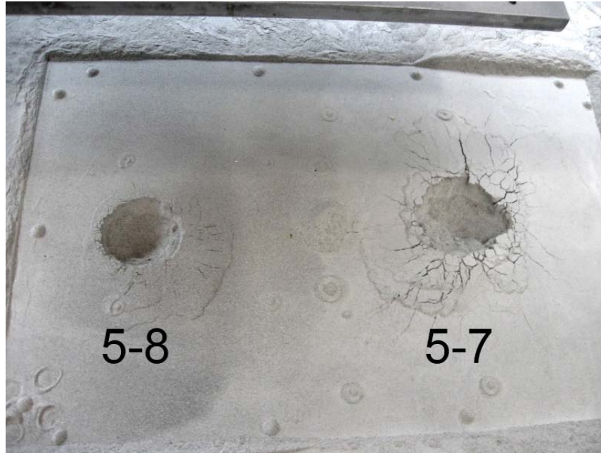
Figure 26.—Comparison of penetrometer holes from runs at vacuum (5-7) and ambient (5-8) conditions.
