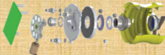
CubeSat-class 50-mm (2") imaging camera/instrument - mirrors and integrated optical-mechanical structures- manufacturing with 3D-printed parts
