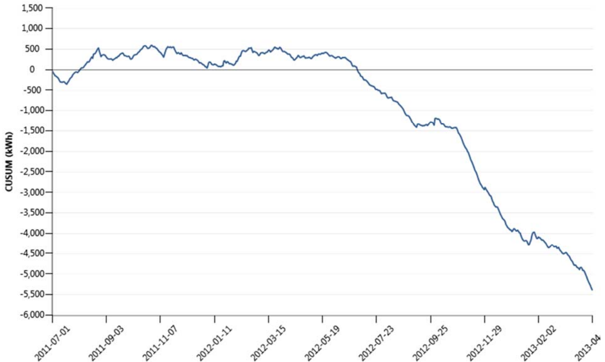
Figure 25. Cumulative sum (CUSUM) of daily electric consumption for a NASA Langley building using the time series from July 2011- July 2012 as the baseline. This CUSUM indicates a net energy savings of approximately 5,500 kWh over the period from August 2012-March 2013. 10
