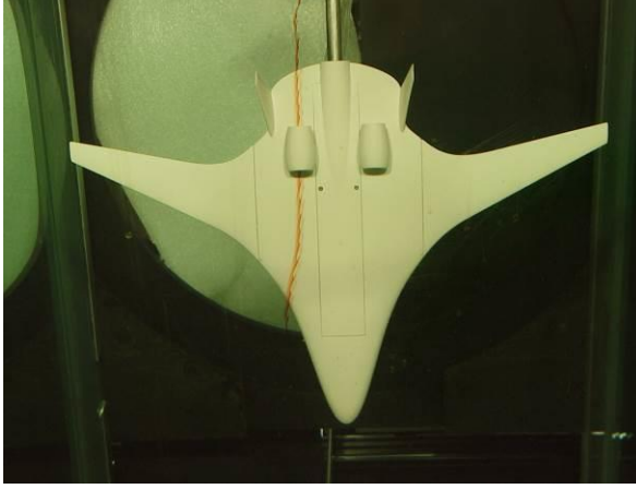
Figure 7. Flow visualization with dye wand over center body at 10° angle-of-attack and 0° sideslip.
