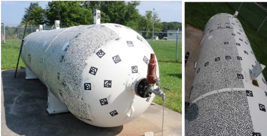
Figure 7.2.3.3-4. Two Views Depicting Placement of Digital Targets on Pressure Vessel
