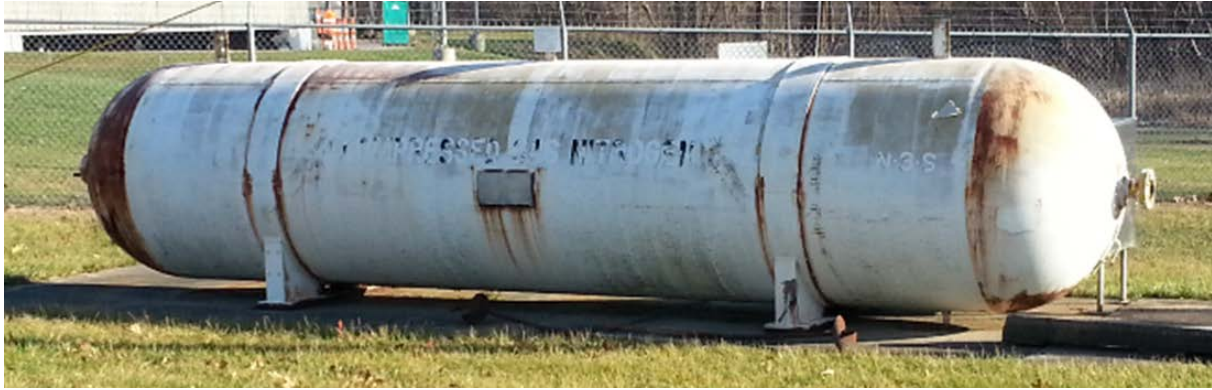
Figure 7.2.3.1-1. Pretest View of PV0236 (vessel measures 52-inches ID × 24 feet long, has an internal volume of 306 cubic feet and a design pressure of 2,800 psig, has a layered shell construction, and was fabricated in 1959)
