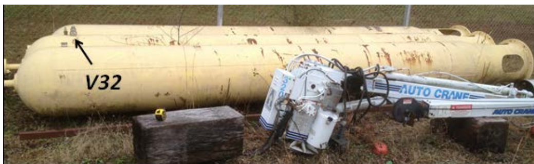
Figure 7.2.1.1-1. Vessel V0032 before Sectioning, Shown with Sister Vessels V0030 and V0035
