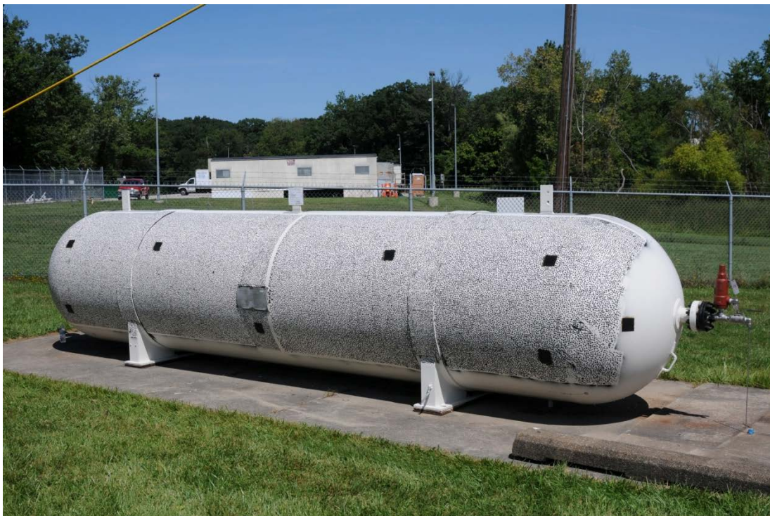
Figure 7.2.3.3-3. Pressure Vessel with Completed Dot Pattern
