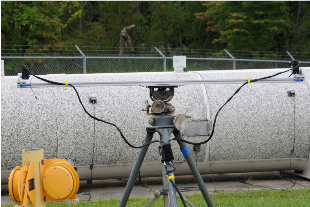
Figure 7.2.3.3-5. Aramis Camera Pair in Test Configuration (note acoustic sensors on vessel)
