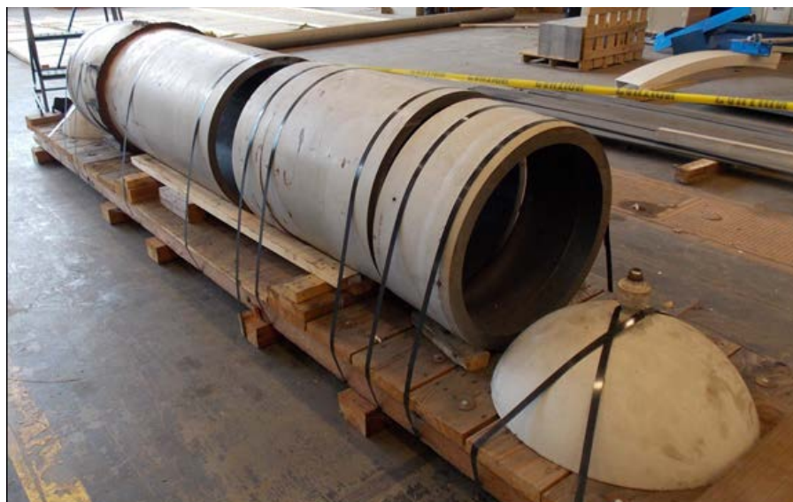
Figure 7.2.1.1-2. Vessel V0125 Shown after Sectioning
