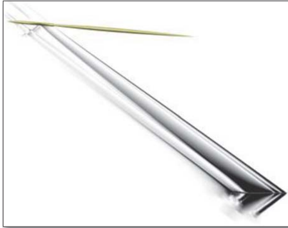
Figure 21. Contours of density-adjoint ( |\psi_0| , white 0, black 0.012) on symmetry plane
