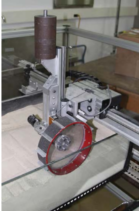
Figure 2.—Wheel test rig used with soil optical flow technique.
