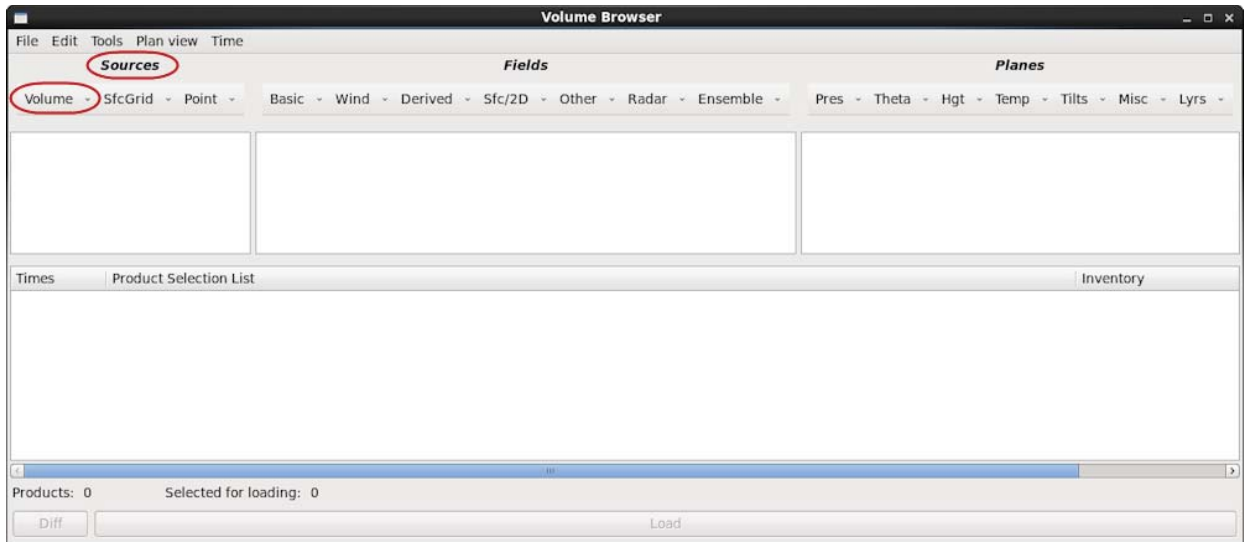
Figure 15. Volume Browser window in CAVE. The AMU WRF-EMS is selected by clicking the Volume drop-down menu under Sources.
