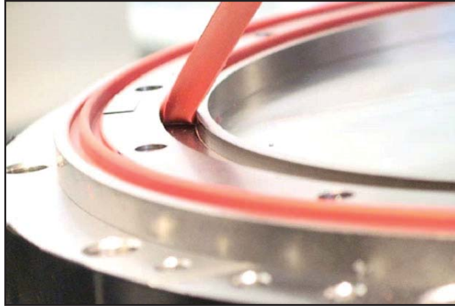
Figure 15.—Gask-O-seal bulb being pulled out of its retainer during bond strength test.
