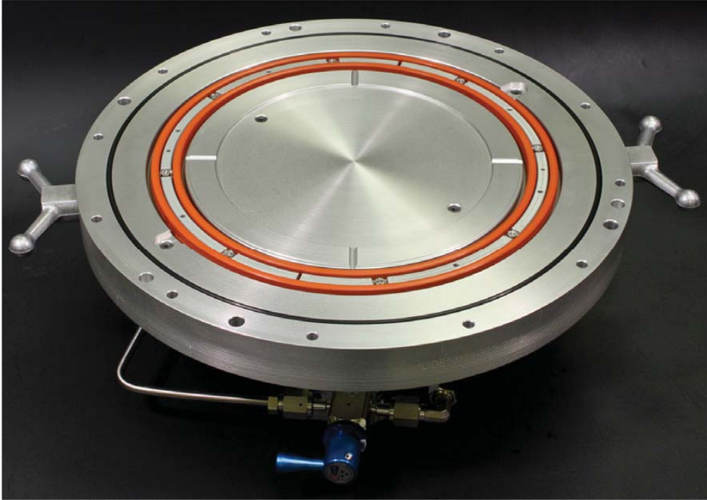
Figure 12.—Medium-scale seal leak test fixture. (Note: Top of test fixture is not installed.)
