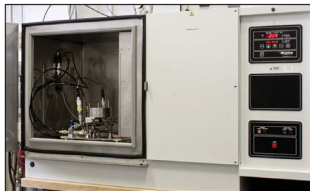
Figure 9.—O-ring leak test fixture installed in environmental control chamber.
