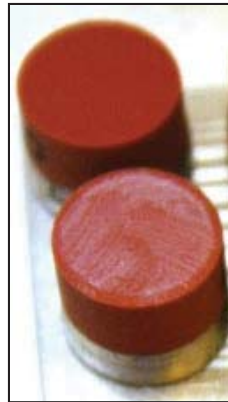
Figure 10.—Small-scale, cylindrical “button” test specimens.
