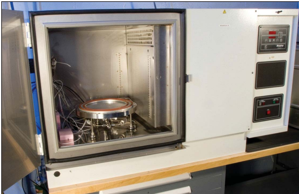
Figure 13.—Medium-scale seal leak test fixture installed in environmental control chamber.
