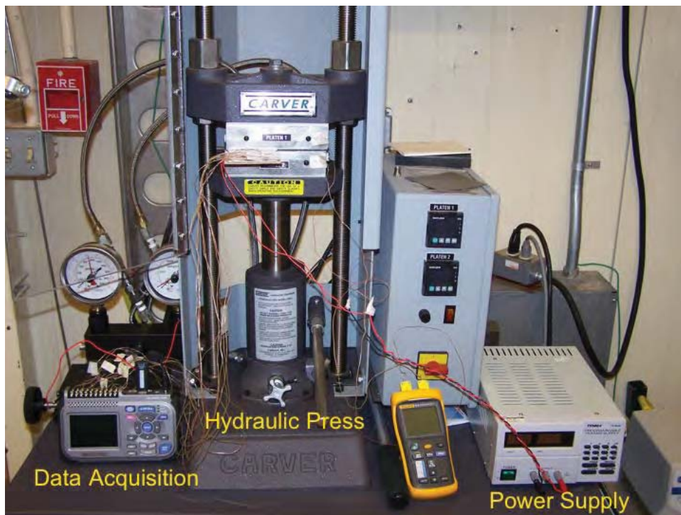
Figure 5.1.—Hydraulic Press Heat Pipe Test Setup
