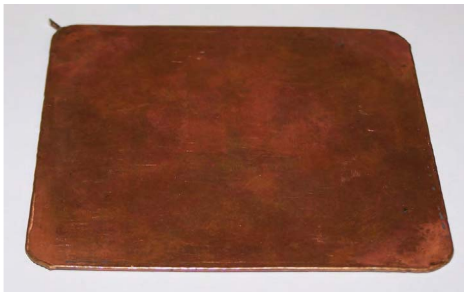
Figure 2.13.—Copper Flat Plate Heat Pipe
