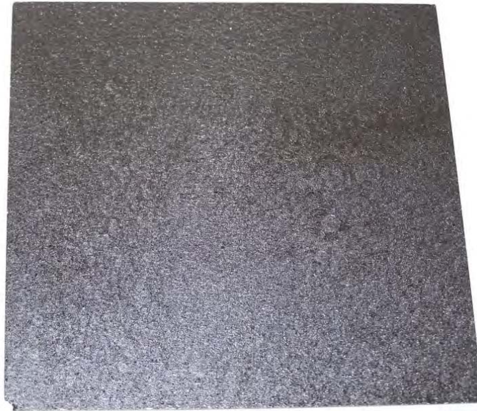
Figure 2.1.—TPG Sample (9.8- by 9.8- by 0.05-cm)
