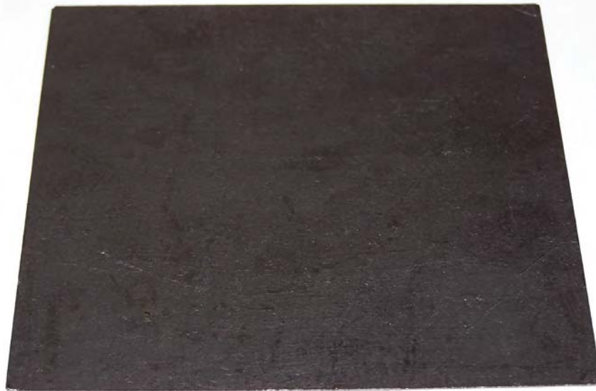
Figure 2.9.—Carbon Painted TPG Plate (9.8- by 9.8-cm)
