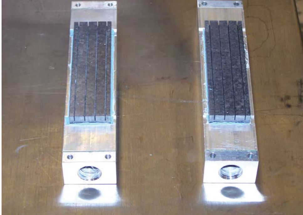
Figure 6.4.—D5506 LCP and Aluminum Cooling Manifolds
