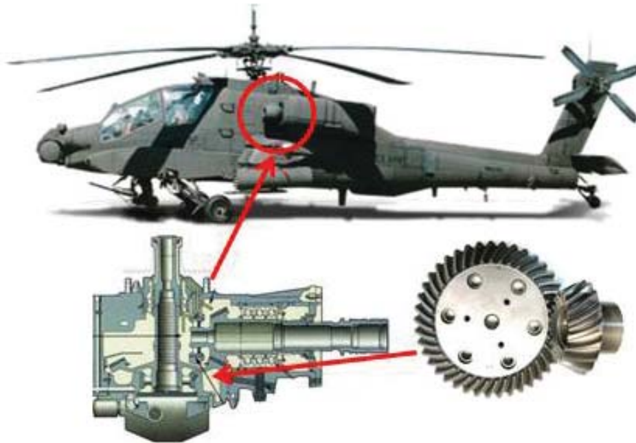
Figure 1.—Location of spiral bevel gear set in helicopter
