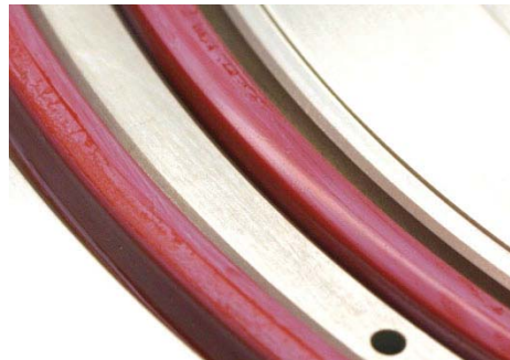
Figure 11.—Coated Medium-scale seal –0283 after adhesion testing at -8\text{ }^{\circ}\text{C} (8 hr dwell) and then 25 more times at room temperature (1 min. dwell on each cycle).
