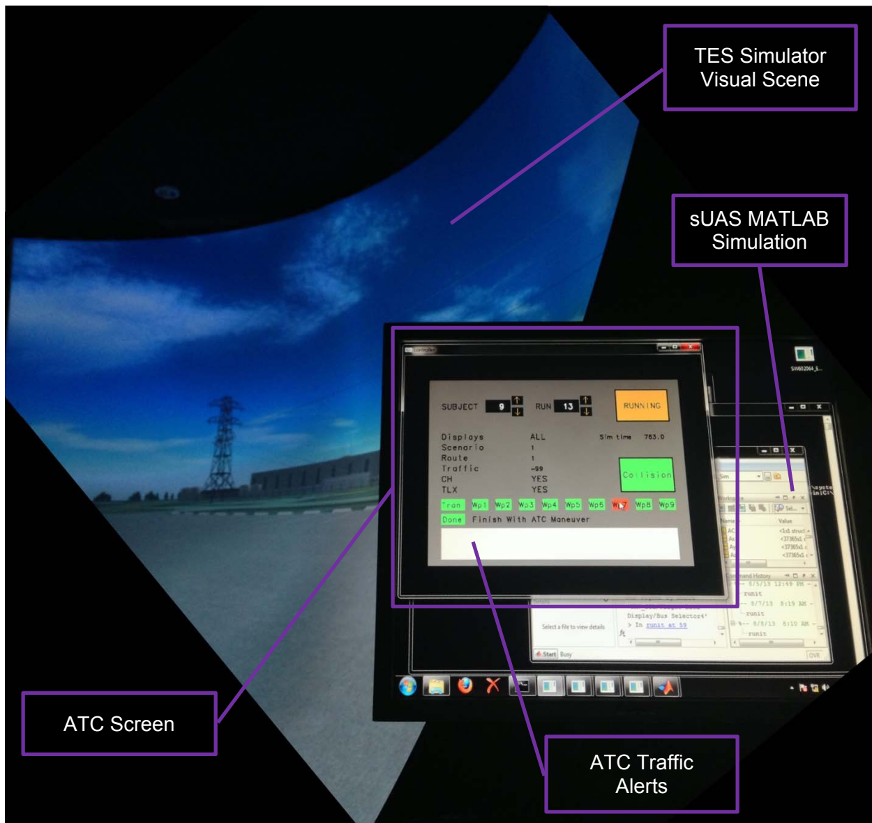
Figure 6 – ATC Alerts Pop-Ups and Test and Evaluation Simulator
