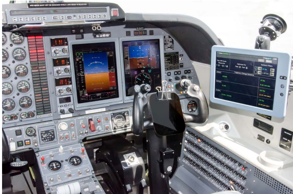
Figure 7. Test-bed cockpit. The EFB is mounted on the right-side windshield.
