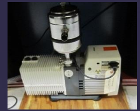
Vacuum ops down to 5 \times 10^{-6} Torr
