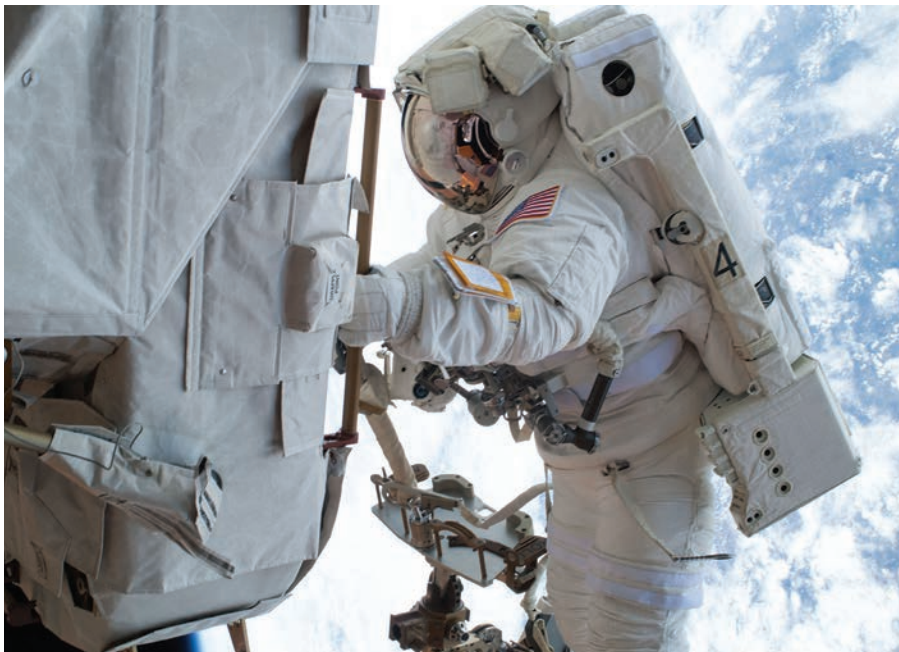
NASA astronaut Mike Hopkins works to change out a faulty water pump outside the International Space Station in December 2013. To dissipate body heat that accumulates in his spacesuit, an undergarment circulates chilled water through tubes pressed against his entire body.
