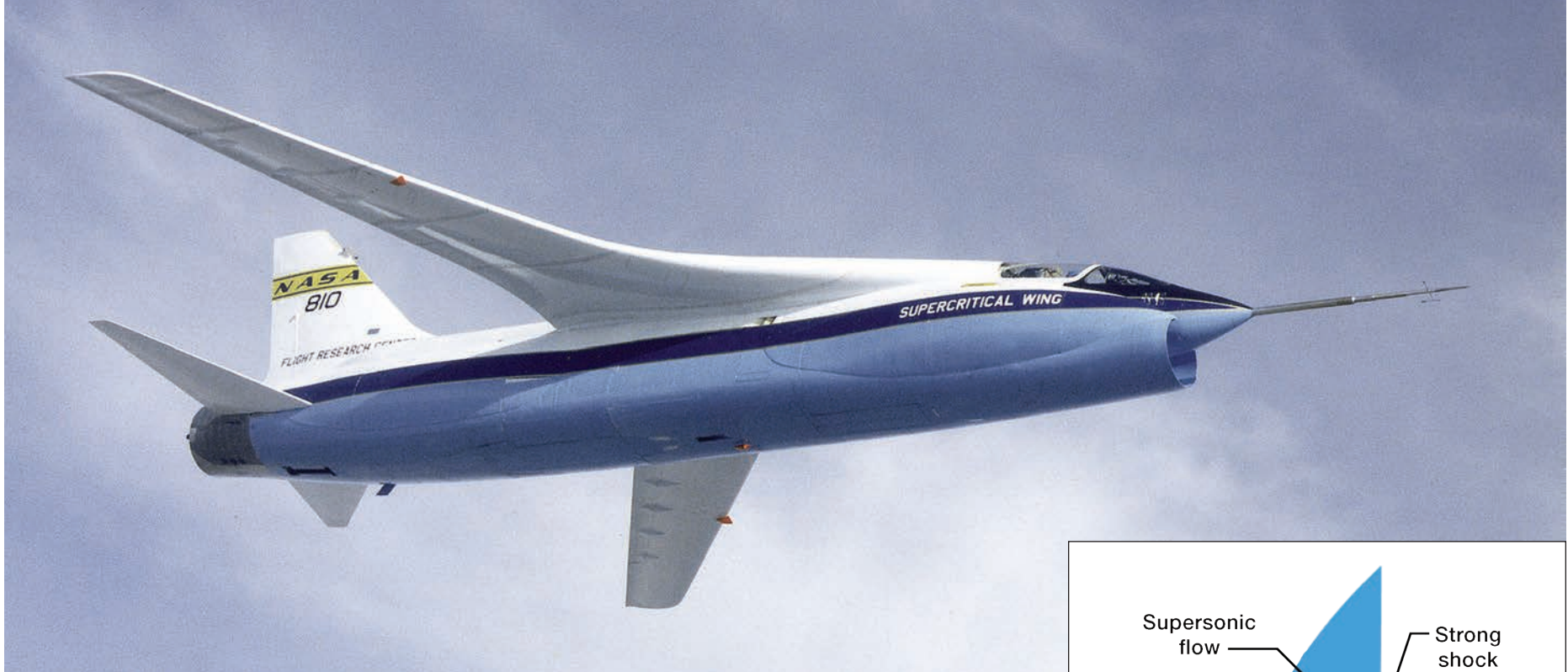
The first aircraft used to test supercritical wing designs was a modified Vought F-8 Crusader provided by the US Navy.
