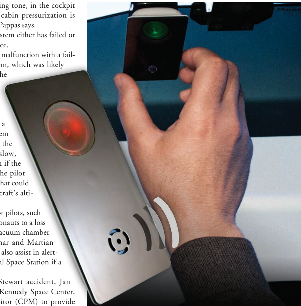
Aviation Technology Inc.'s Alt Alert cabin pressure monitor uses a flashing, red light combined with either advisory chirps or sustained alarms, depending on the seriousness of the situation, to alert pilots and crewmembers to a loss of cabin pressure. The device can be secured to a visor with a clip, but it can also use a suction cup to attach to a window, or Velcro for mounting on an instrument panel.
