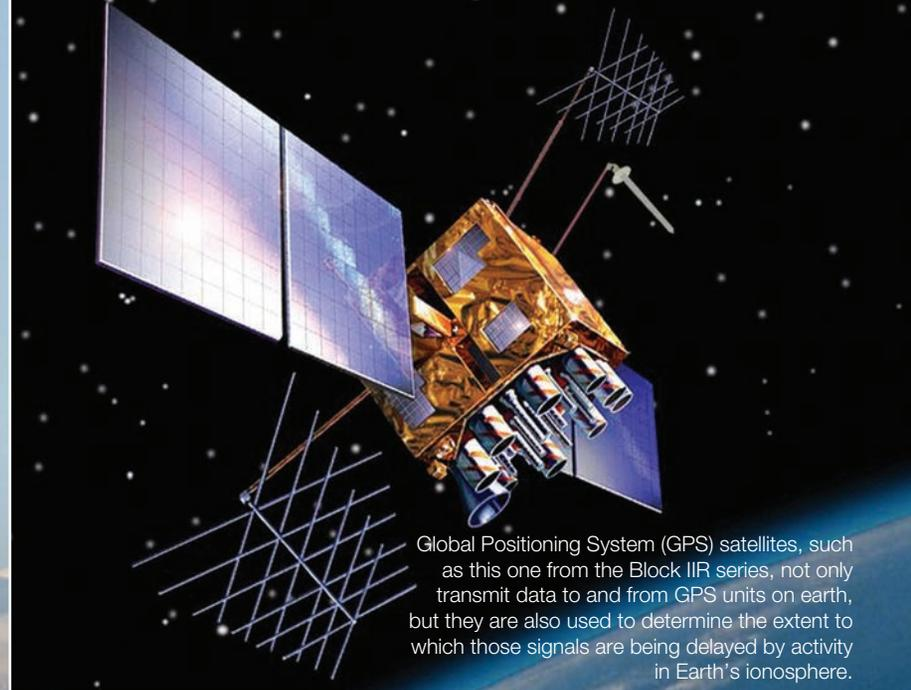
Global Positioning System (GPS) satellites, such as this one from the Block IIR series, not only transmit data to and from GPS units on earth, but they are also used to determine the extent to which those signals are being delayed by activity in Earth's ionosphere.
