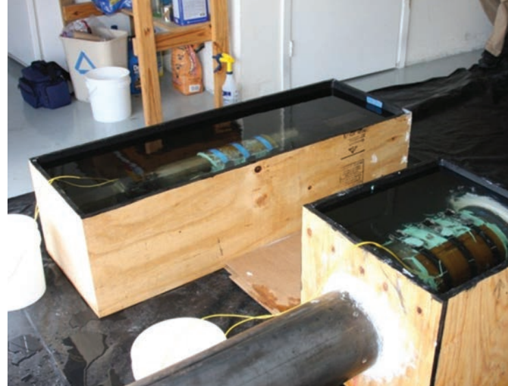
Pictured here are two tests of ATI's clamps in a NASA lab at Johnson Space Center. On the left, a proprietary coating uses friction to keep the clamp in place. On the right, a special adhesive works even underwater to bind clamps to pipes.
