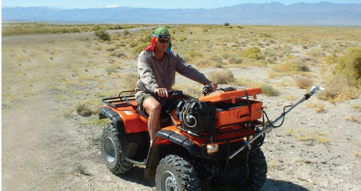
One of Ocean Optics' NASA-improved spectrometers is attached to an all-terrain vehicle, which is utilizing the instrument for analyzing upwelling and downwelling types of radiation in the desert. The temperature- and shock-resistant properties of the spectrometer prove vital in such a rugged environment.
