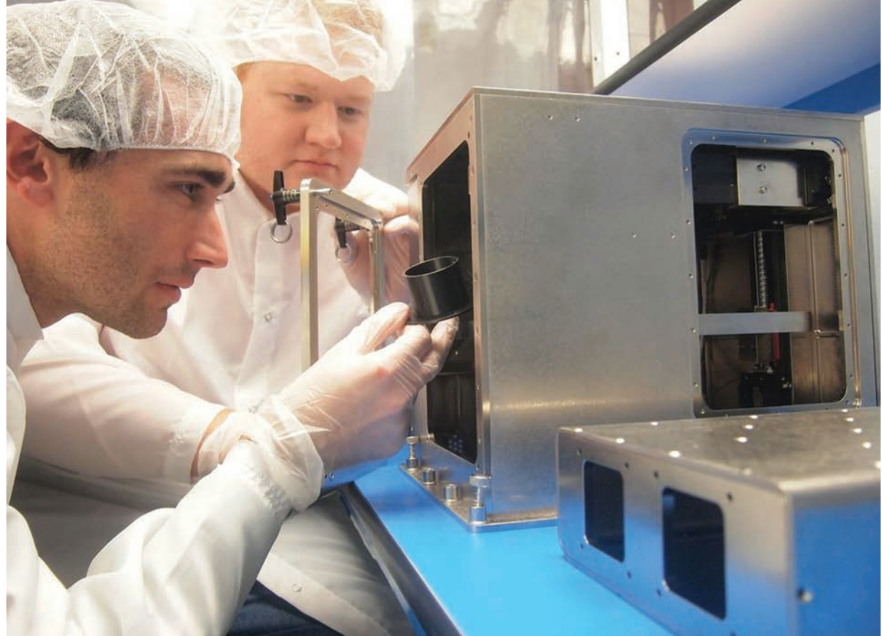
In the Made In Space “clean room,” Chief Technology Officer Jason Dunn pulls a sample part from the company’s prototype for a 3D printer that can operate in microgravity, as lead engineer and director of research and development Michael Snyder looks on.
