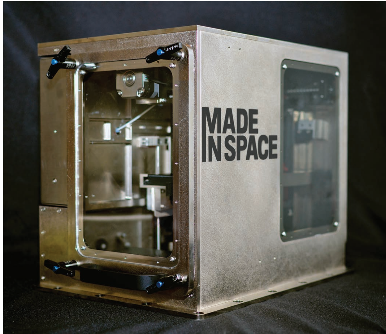
The prototype for a 3D printer capable of operating in microgravity, created by Made In Space with the help of a couple of Small Business Innovation Research contracts with NASA's Marshall Space Flight Center, is slightly smaller than the one the company will create for installation aboard the International Space Station.
