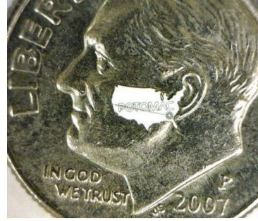
This example demonstrates the company's ability to laser micromachine polyethylene terephthalate, a thermoplastic polymer, at micron scale.
