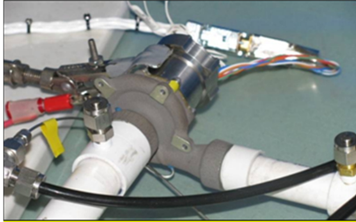
Figure 5. Fan Installed for Testing (Updated Photo due for final paper)
