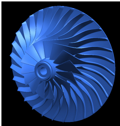
Figure 58.—HECC impeller geometry has 15 main blades and 15 splitter blades. The picture on the right shows the rounded trailing edges and fillets.
