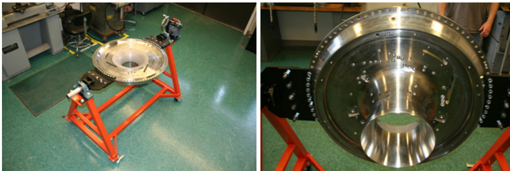
Figure 93.—Custom built fixture for holding the shroud, and for assembling the stationary parts
