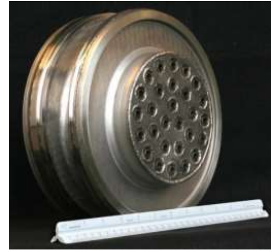
28 element Inconel 625 fuel injector built using SLM process
