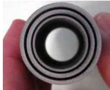
Reentrant titanium tube made by AM for a cryogenic thermal switch for the ASTRO-H Adiabatic Demagnetization Refrigerator
