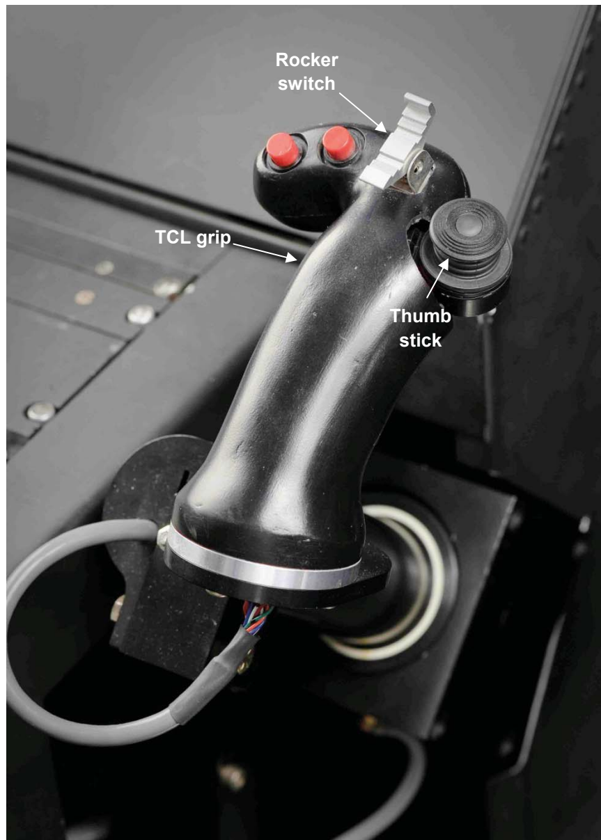
Figure 18. Thrust Control Lever Grip. Center rocker switch controls discrete nacelle movement. The thumb stick is a two-axis proportional controller. Used with TRC, the stick provides an alternative to center stick inputs for longitudinal and lateral speed control. In ACAH, the thumb stick controls fore and aft nacelle rate, proportional to control displacement, up to a maximum of 7.5 deg/s.
