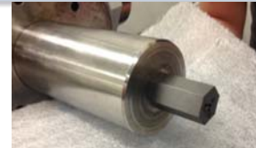
Above and Left: Extrusion samples using carbon-matrix/Ha blend .75" across flats, .125" coolant channels
