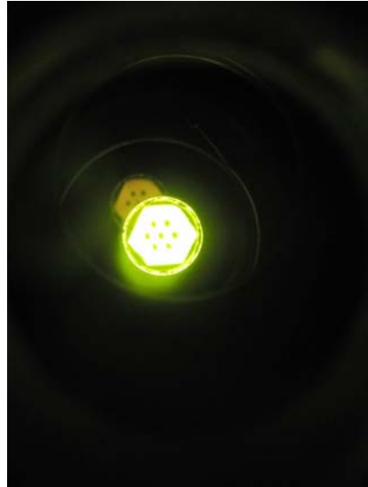
Initial Testing of Short W/UO 2 Element Segment
