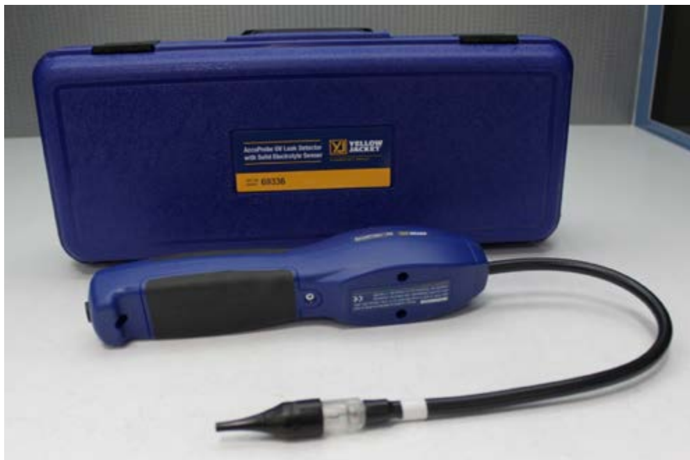
Figure 17. Hydrocarbon leak detector.
