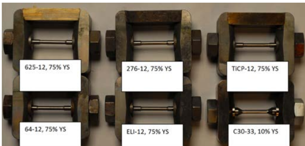
Figure 3. Representative assembled and loaded stress corrosion specimens before test.
