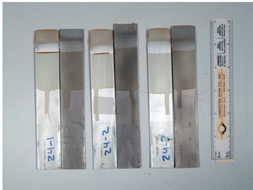
(e) FM 300-2, 393 K Cure (Condition 24), Room Temperature Test
