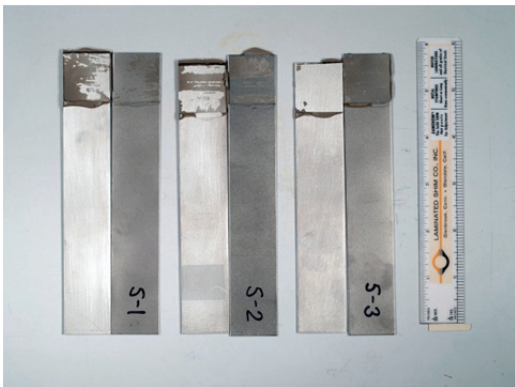
(a) EP30HT-LO, With Silver, RT Cure + 343 K Post Cure Treatment (Condition 5), Room Temperature Test
