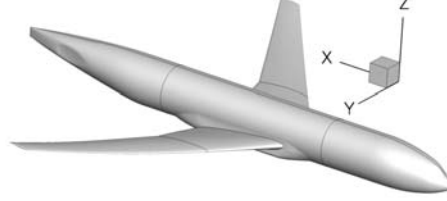
Figure 3: FUN3D body coordinate system.
