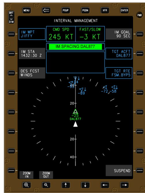
Figure 1. Side-mounted electronic flight bag (EFB) and Flight Deck-based Interval Management (FIM) application.
