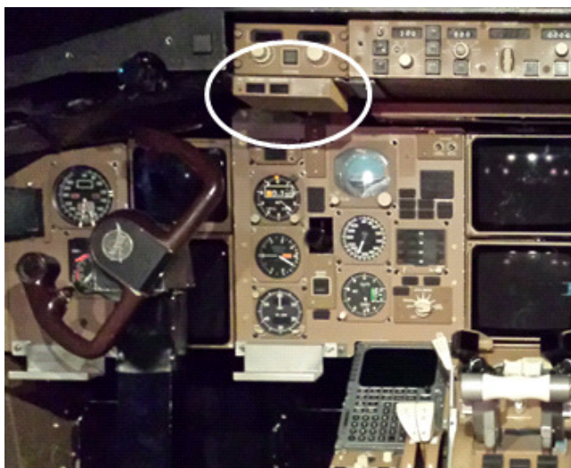
Figure 2. ADS-B guidance display (AGD) presenting target and error speed values.
