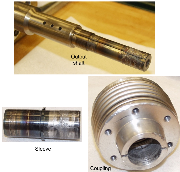
Figure 37.—Output shaft coupling failure.
