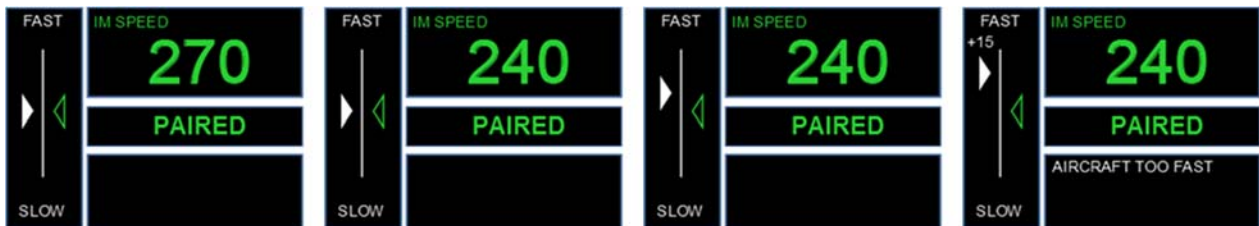
Figure 15. Sequence of FAST/SLOW indicator during IM speed change.
