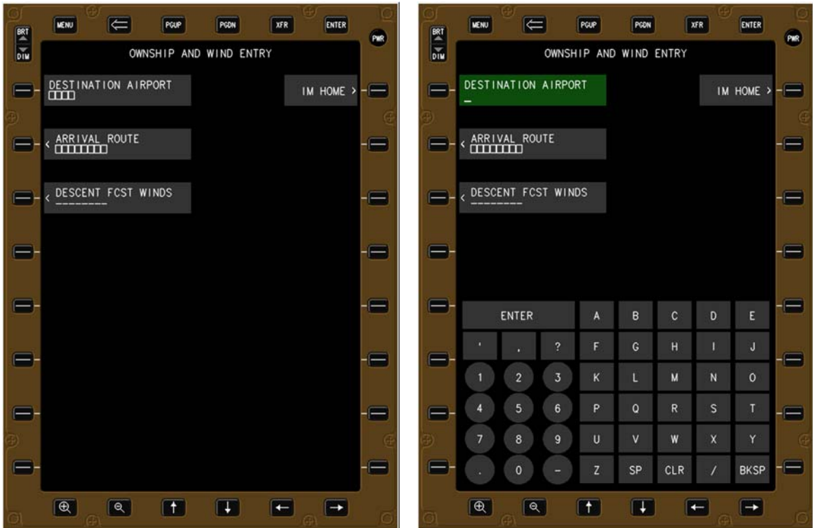
Figure 63. Data field selection in right EFB is not seen by left EFB.
