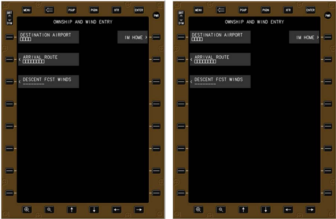
Figure 62. XFR button to change left EFB to same page as right EFB.
