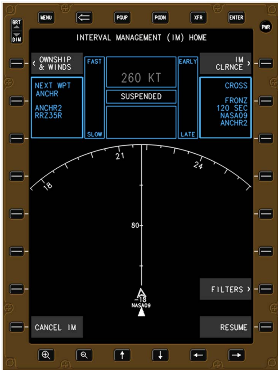
Figure 78. EFB in SUSPENDED-AVAILABLE state.
