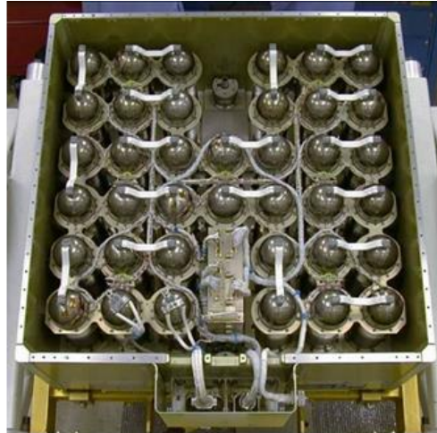
NiH 2 Battery ORU ©2007 Space Systems Loral
