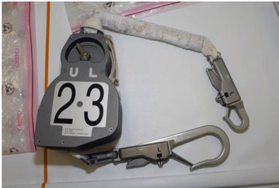
Figure 7.11-1. Safety Tether showing the Insulating Fabric Section at the End
