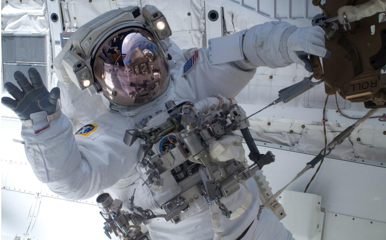
Figure 7.11-2. EMU showing the Fabric section of the Safety Tether and how all the Anodized Rings are Covered by the Suit Fabric
