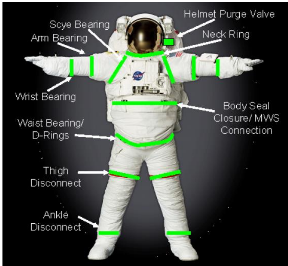
Figure 6.3-9. EMU Suit External Metal Locations [ISS-NCR-232F Attachment 5, 2012]
