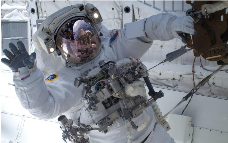
Figure 7.9-3. Suited astronaut: EMU upper part (picture source unknown). Some details of wrist, EMU tether lower right and equipment/tool tether (right) shown.
