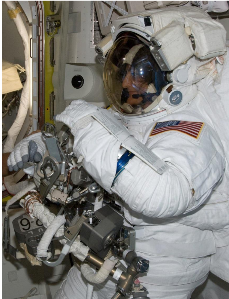
Figure 7.10-2. Example of an exposed section of the stainless steel wrist bearing ring directly above the blue anodized ring [Roeschel, 2013]. Normally both rings are covered by suit fabric.
